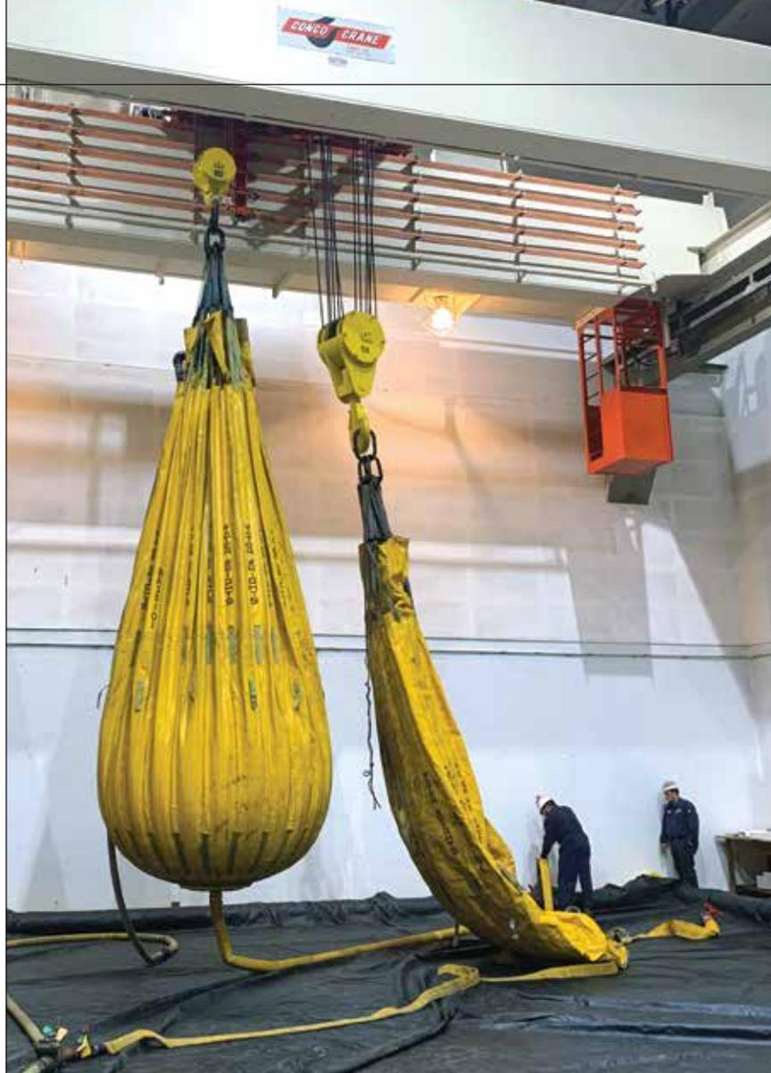
10-ton load testing. 2,400 gallons of water were filled into a large tote for a 10-ton test.
